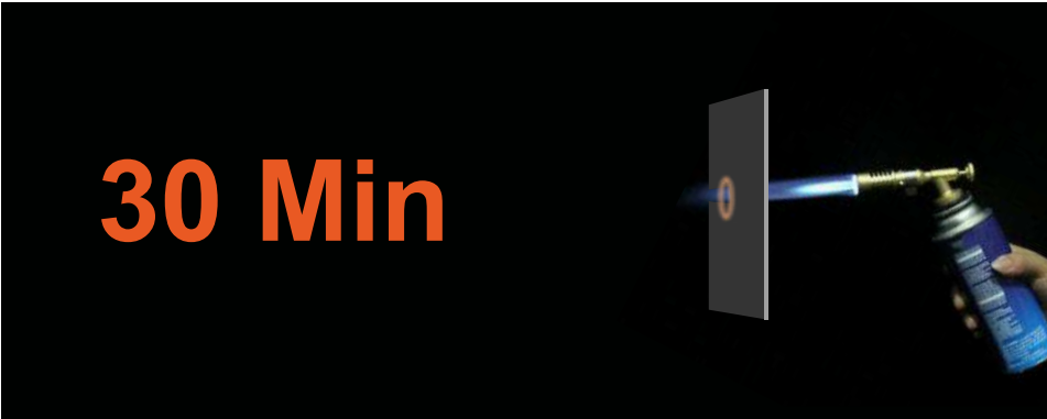
A2 MINERAL CORE - ACP PANEL - FIRE PENETRATED IN 30 MINUTES
