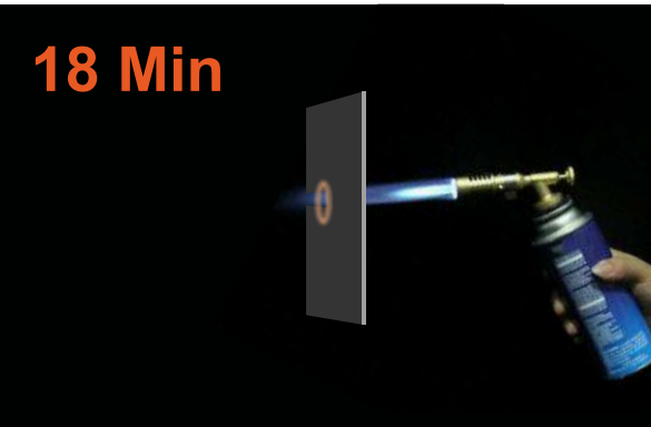
B CORE - ACP PANEL - FIRE PENETRATED IN 18 MINUTES
